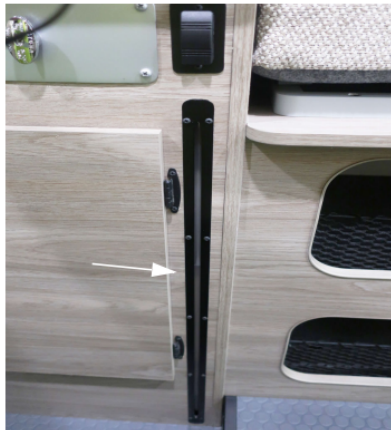
Tank water level indicator- depress button above to view water level in low light conditions. Can be left on to be used as a night light. (located on sink cabinet) -Typical View
