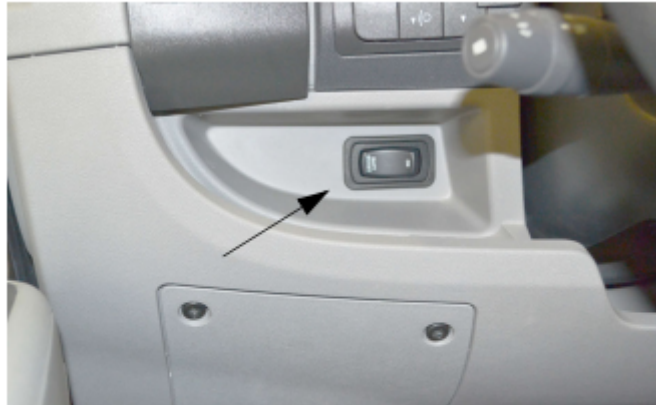
Battery Boost Switch (Located on lower dash area) • Press and Hold in the ON position while turning ignition key for emergency starting power. -Typical View
