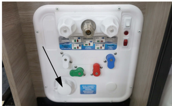
Tank Fill Inlet (Located behind the passenger rear door) -Typical View
