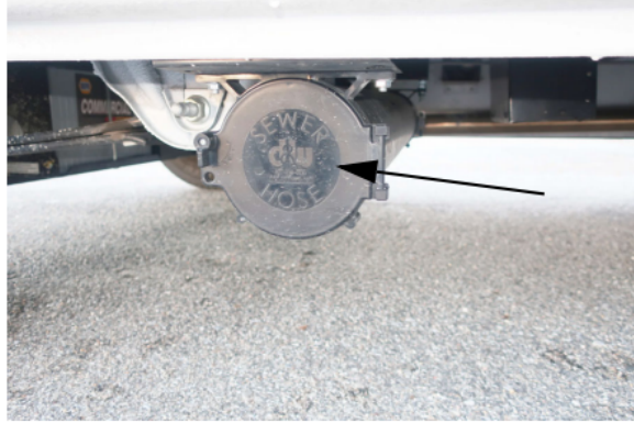
Sewage Drain Hose (Located under the sliding door area) -Typical View
