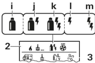
The “Select energy mode” menu is displayed only if a furnace with electric heating elements is connected (Trauma Combi eco plus or Trauma Combi (D) comfort plus).
