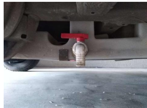
Grey water tank opening/closing tap
